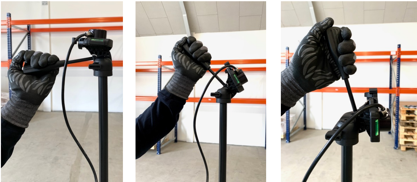
Figure 7: Examples of different sensor directions when measuring to locate hotspots.
