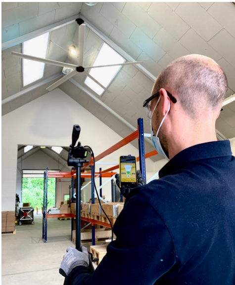
Figure 6: Setting the height of the sensor head to a standard 183 cm or acceptable height for the tasks that are performed in the room.
