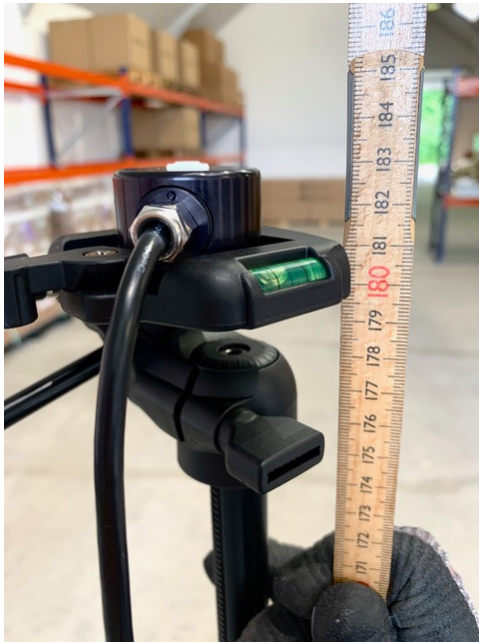
Figure 6: Setting the height of the sensor head to a standard 183 cm or acceptable height for the tasks that are performed in the room.
