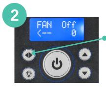
The home screen will automatically appear. To go to fan settings, press this button and hold for 4 seconds.
