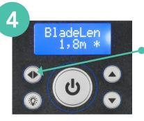
You are now in Blade Length settings. As a standard, the blade length is set to 1,8 meters, as indicated by the star. Press the shift button to change blade length setting. Continue until you reach the correct fan size.
