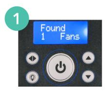
When connecting the controller using the CAT 5E cable, this screen will appear after a few moments. This screen indicates that a fan is found and is only shown briefly.
