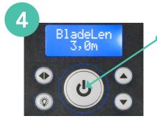
When you reach the correct fan size press the on/off button to save.
