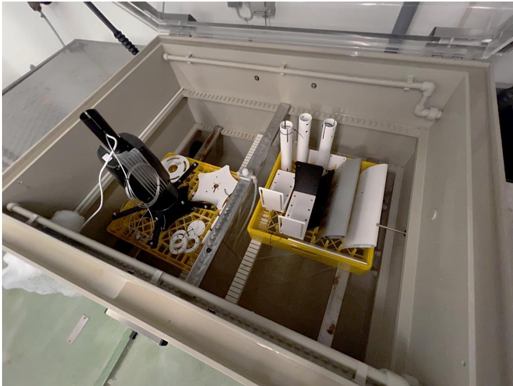
Photo 5 Test set-up salt mist chamber.
