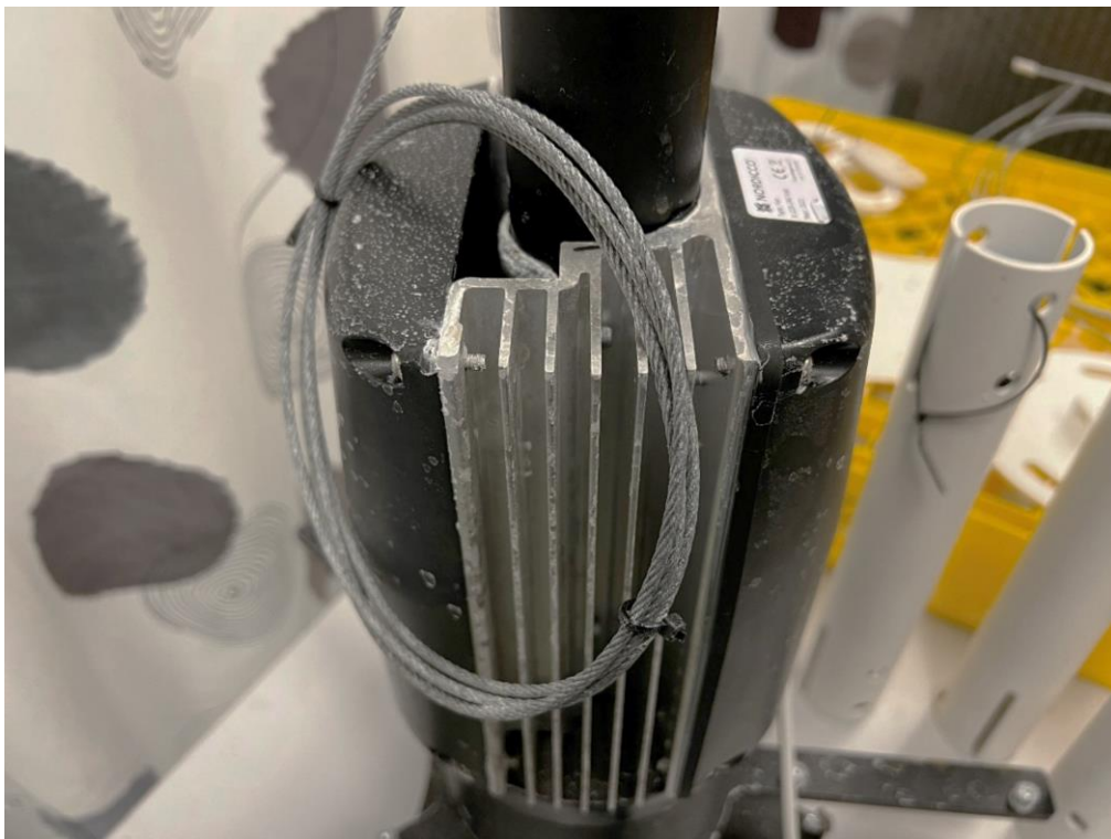
Photo 6 Visual inspection (fan). Slight oxidation on aluminium heat sink.
