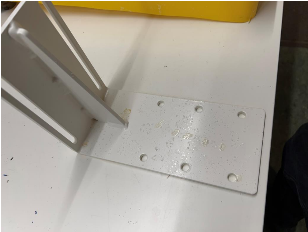
Photo 17 Visual inspection. (Wood/concrete mount P/N: 20032) slight coloration on repaired cracks, otherwise no change.
