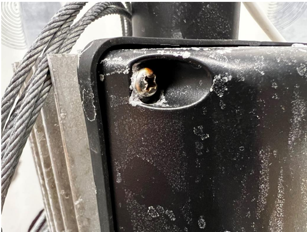
Photo 8 Visual inspection (fan). Corrosion on screw for the lid.
