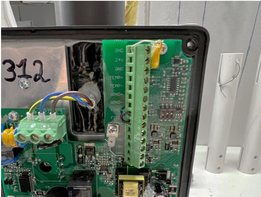
Photo 36 Visual inspection. IPX5. No ingress of water observed inside the enclosure of the test object.
