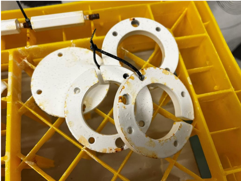
Photo 15 Visual inspection. (Cable retainers P/N: 20007 & 20008) slight corrosion along edges and scratches made by the client.
