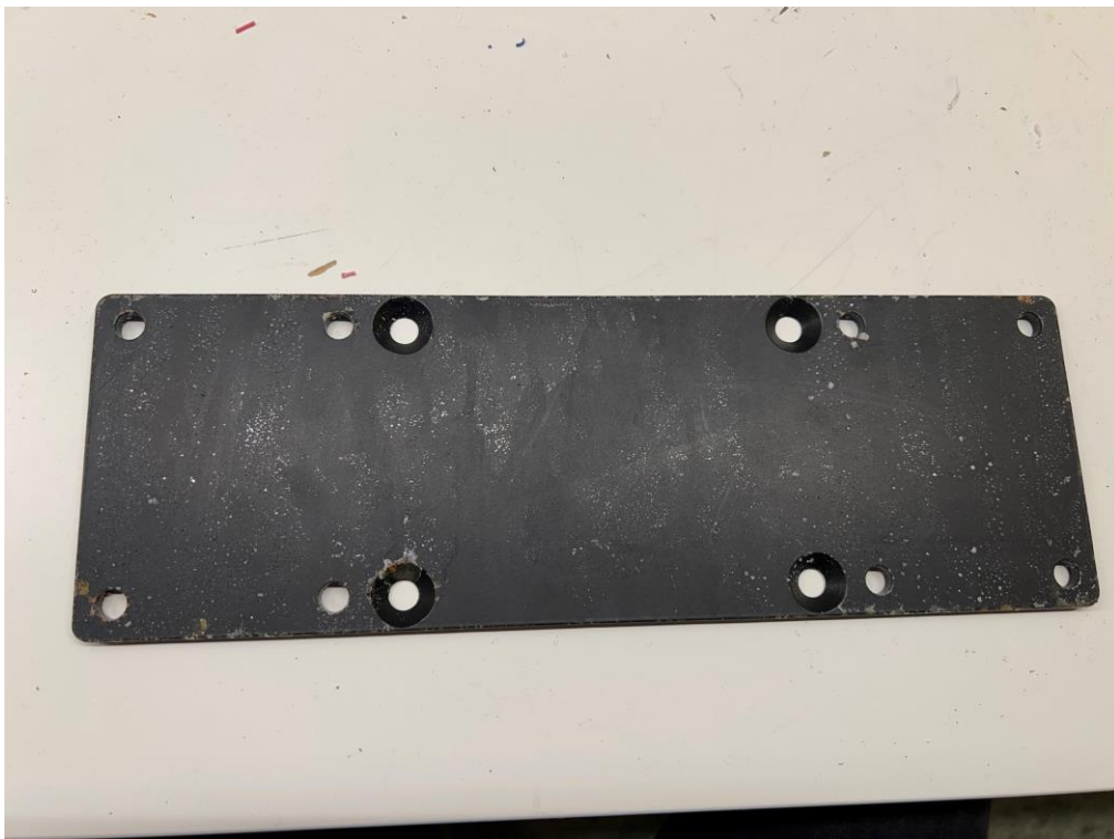
Photo 20 Visual inspection. (Saddle extension plate P/N: 20028) corrosion on scratches made by the client and along edges.
