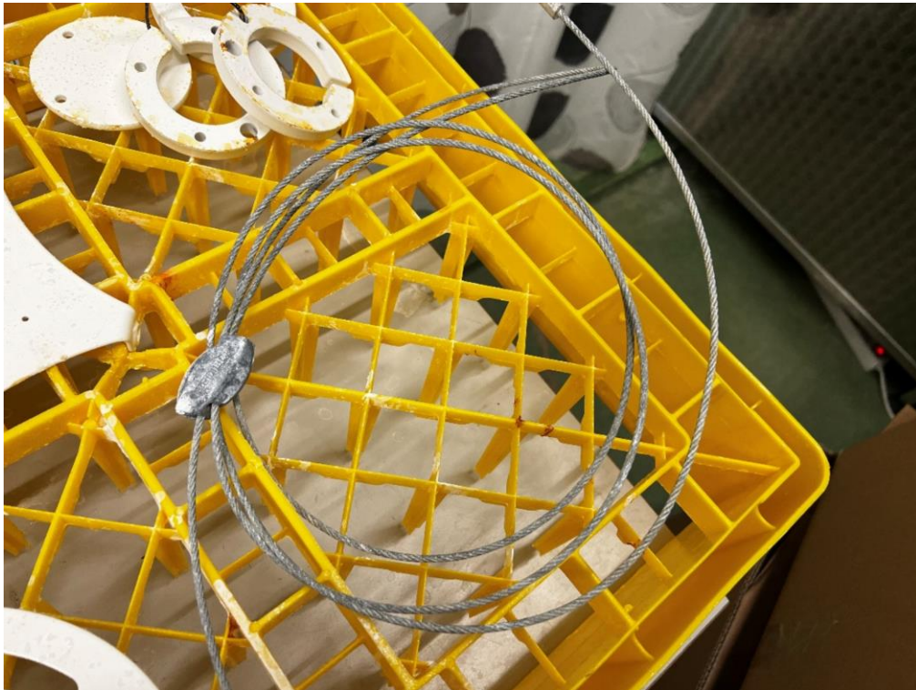
Photo 13 Visual inspection. (Safety wire & Gripple, P/N: 300-104 & 10013). Oxidation and slight corrosion observed.
