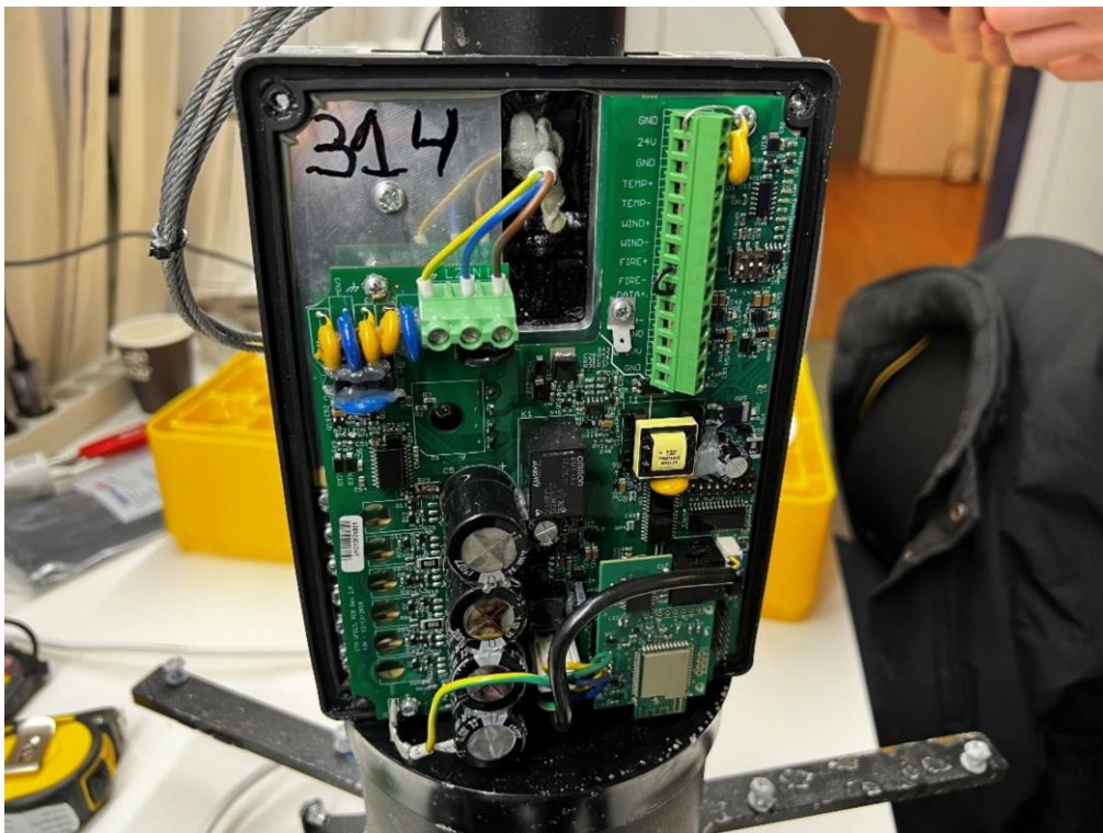
Photo 10 Visual inspection (fan). No signs of corrosion or salt residue inside the test object.
