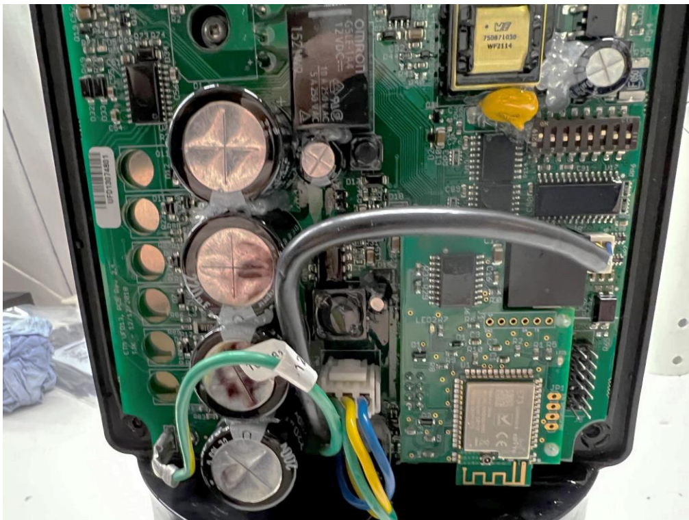
Photo 37 Visual inspection. IPX5. No ingress of water observed inside the enclosure of the test object.
