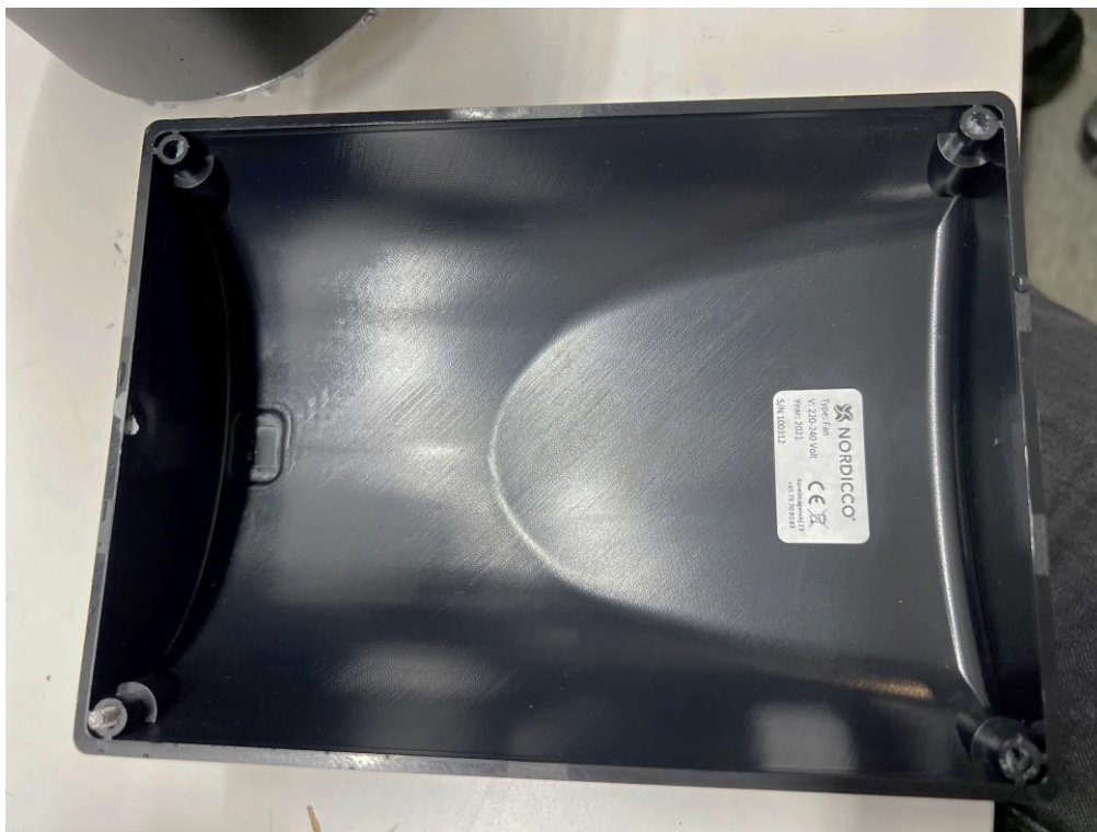
Photo 34 Visual inspection, IPX5. No ingress of water observed inside lid.
