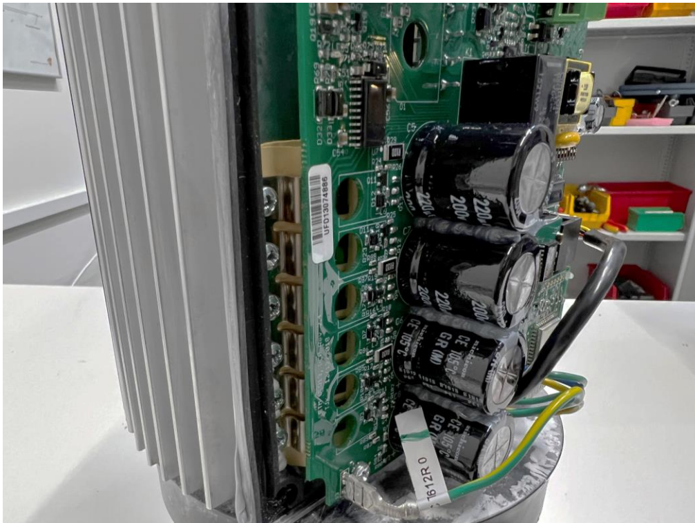
Photo 29 Visual inspection. No ingress of dust observed inside the enclosure of the test object.
