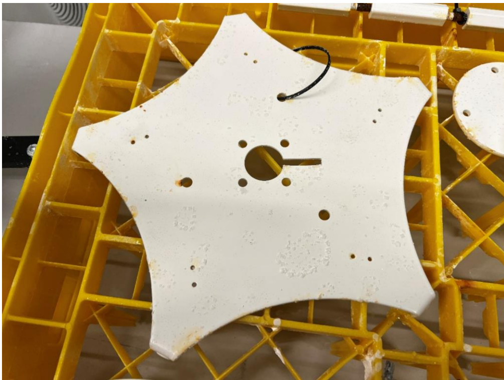
Photo 14 Visual inspection. (Power distributor, P/N: 20009) slight corrosion along edges.
