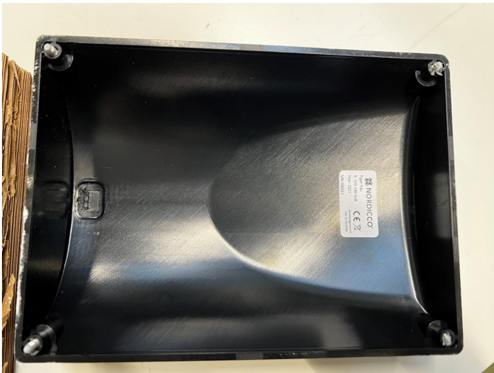
Photo 27 Visual inspection. Lid – no ingress of dust observed.
