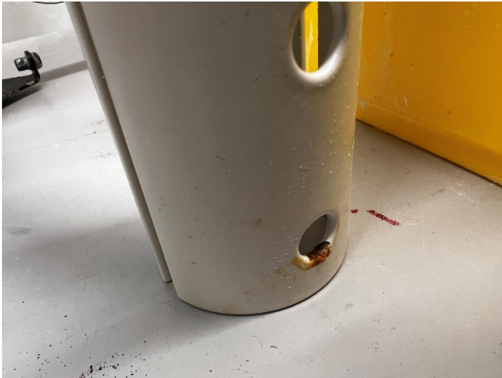
Photo 11 Visual inspection. (Extension tube, P/N: 20003) corrosion on scratch made by the client. Other extension tubes had no changes.
