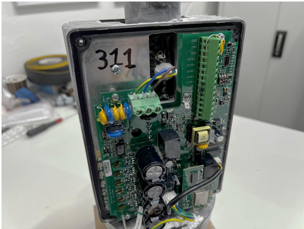
Photo 28 Visual inspection. No ingress of dust observed inside the enclosure of the test object.
