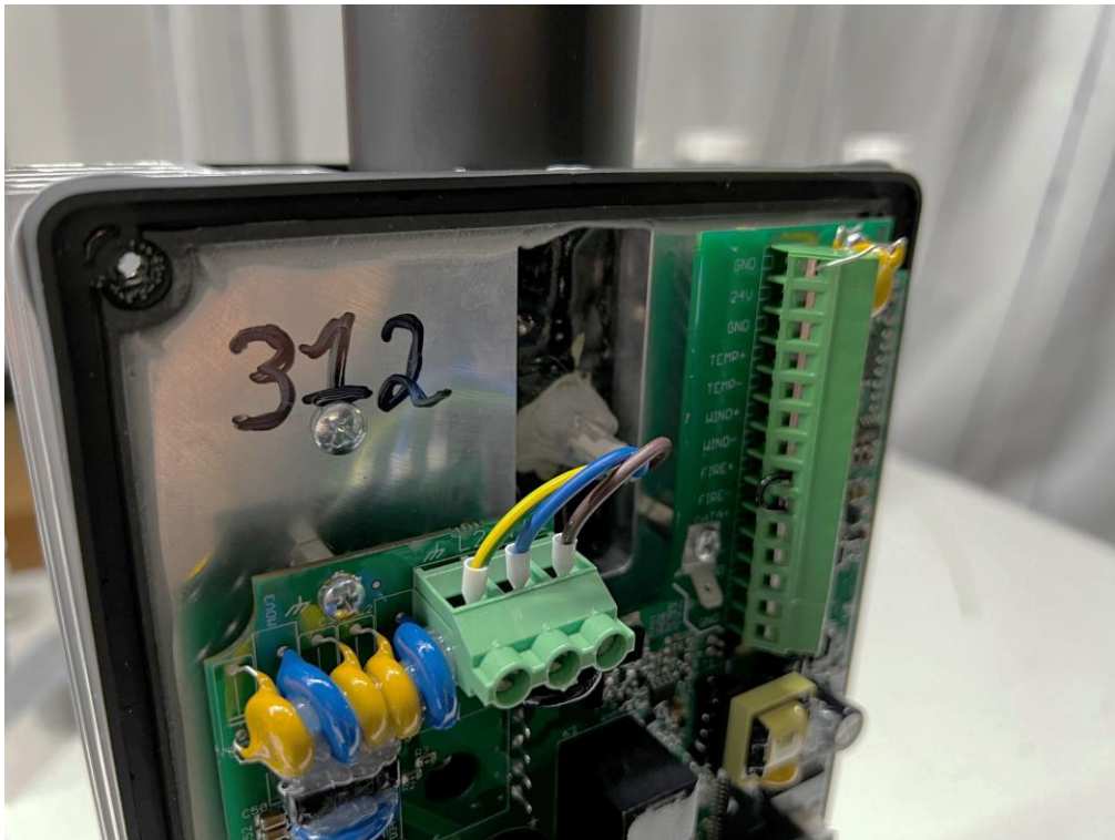
Photo 35 Visual inspection. IPX5. No ingress of water observed inside the enclosure of the test object.
