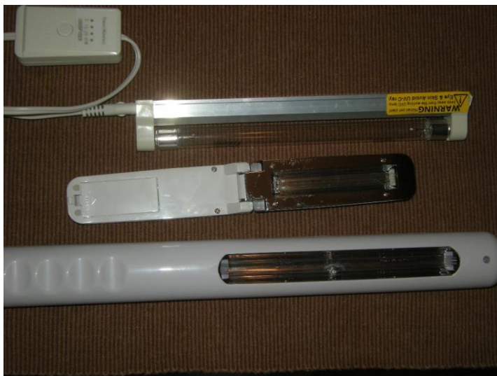
Figure 4-1. Small UV-C mercury lamps and 270-nm LEDs used in hand-held wands are available on the internet (middle and bottom). Small air-space disinfectant units (top) are also sold. (Image courtesy of David Sliney)
